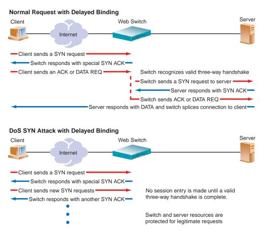
Figure 6-10 Repelling DoS SYN Attacks With Delayed Binding
